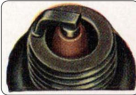
Normal spark plug: Porcelain is light brown in color with slightly dark gray deposits on the edge.
