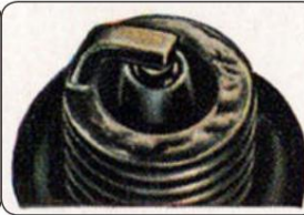
Spark plug too greasy: Greasy black oil deposits. Check engine for broken piston rings too lean and ignition too grease worn cylinder.
