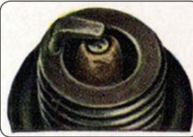
Spark plug worn: Burned out and eaten electrode, and weak spark: install new spark plug.
