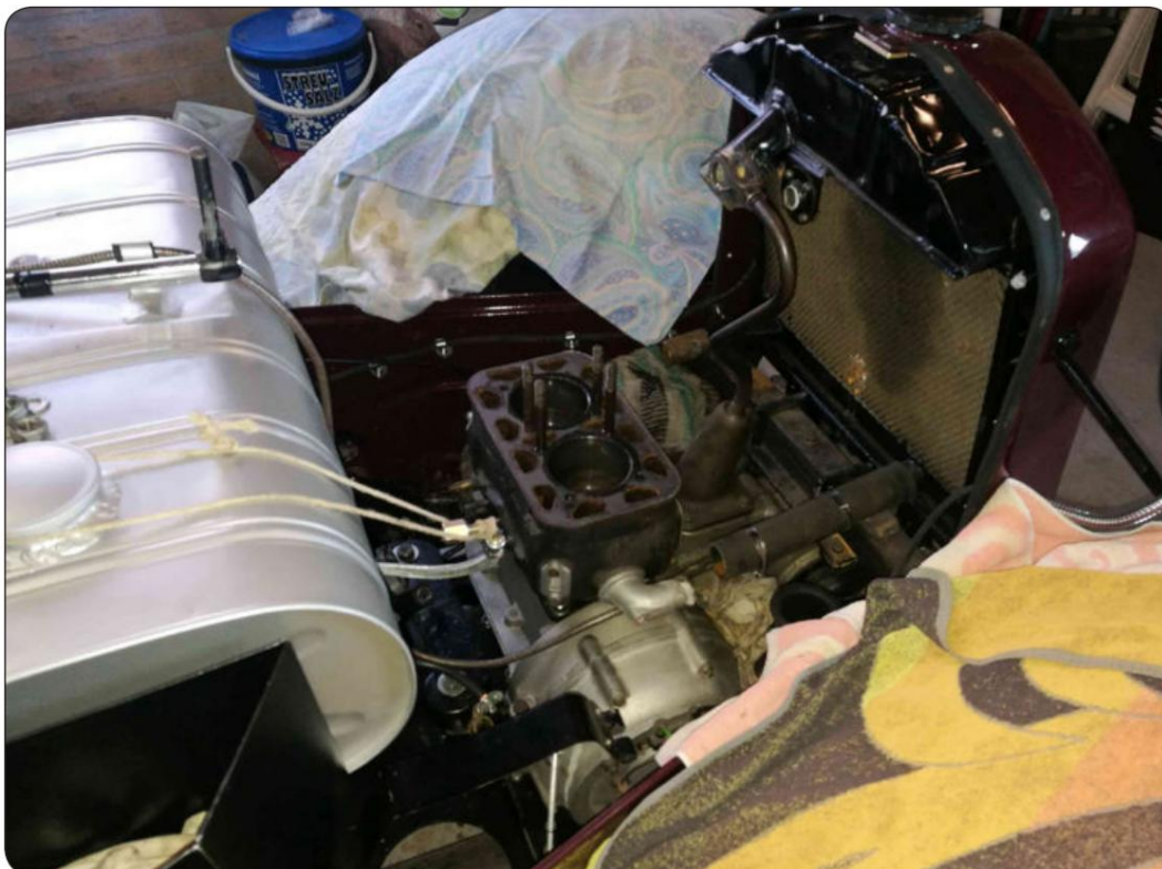
The cylinder head has been removed so that further investigation can be done to determine why the DKW runs poorly.
