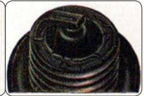
Spark plug rusted: Dry rust deposits: Fuel mixture if necessary. or idling a lot.
